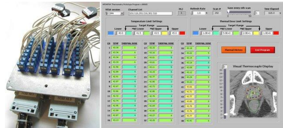
48-channel thermocouple thermometry system for invasive prostate monitoring during Interstitial hyperthermia; From Titania Juang et al., 2009
